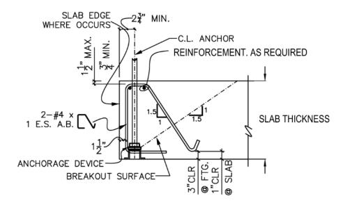
REBAR REINFORCEMENT EDGE EXAMPLE
